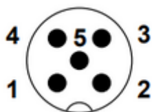
Pin assignment of the Cable connector
